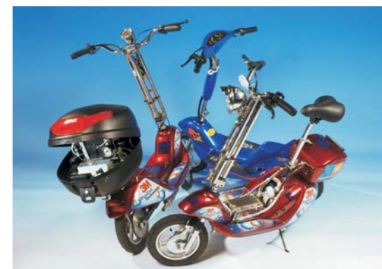
E-scooter with direct and hybrid fuel cell drives
