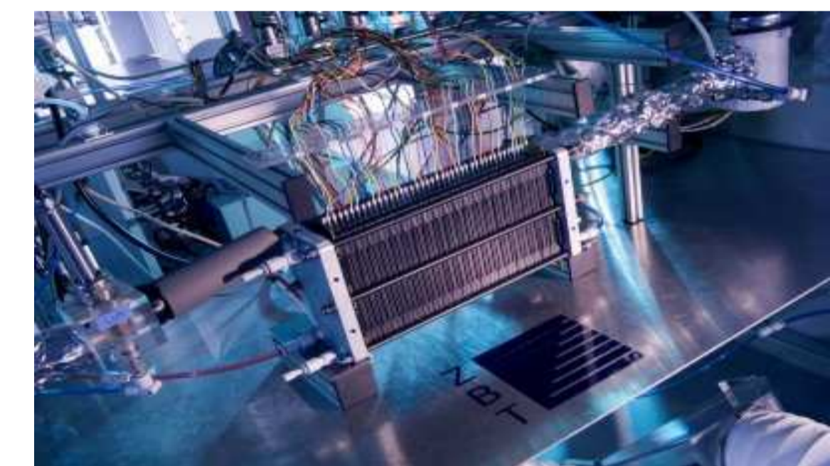
Fig. 9. Typical fuel cell teststand at ZBT
