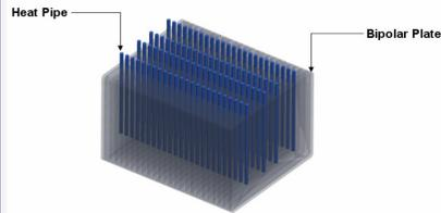
Simplified model of a HT-PEM fuel cell stack assembled with heat pipes
