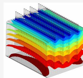
Isothermal surfaces for the first concept at time ( $t=1000$ [sec])
