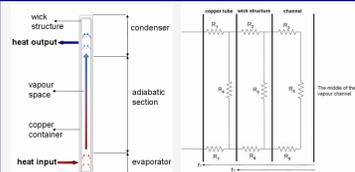
Principle of Heat Pipe and thermal resistance network of a heat pipe
